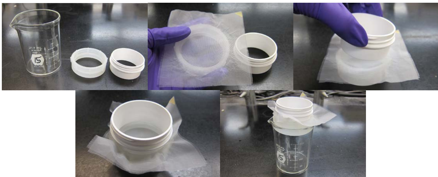
Fig. 17-21: How to set up the sieves with greater than 80 \mu\text{m} fabric.
