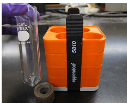
Fig. 7: Glass 40 mL cent. tubes and orange adaptor with black conical rubber insert.
