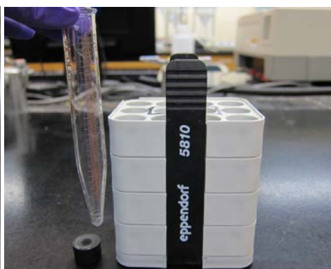
Fig. 5: Glass 15 mL cent. tube and gray adaptor with black conical rubber insert.
