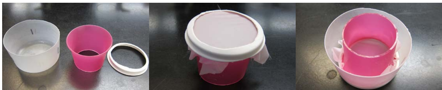
Fig. 22-24: How to set up the sieves with less than 20 \mu\text{m} fabric.
