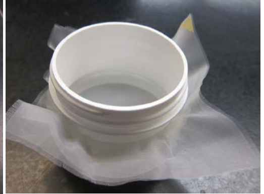
Fig. 12: Sieve system for larger than 80 \mu m fabrics.
