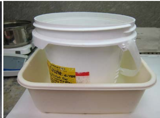
Fig. 15: Bucket used for hazardous waste neutralization in secondary containment tub.
