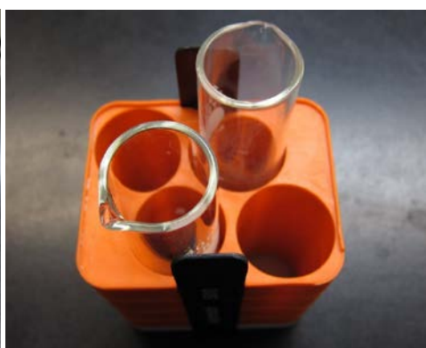
Fig. 8: The two most central positions are the only ones that can be used with the vapor caps.
