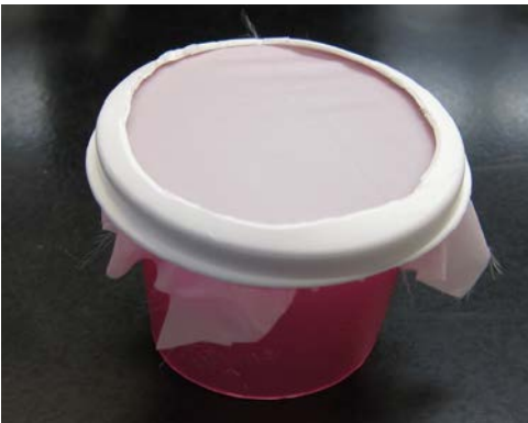
Fig. 13: Sieve system for smaller than 20 \mu m fabrics.
